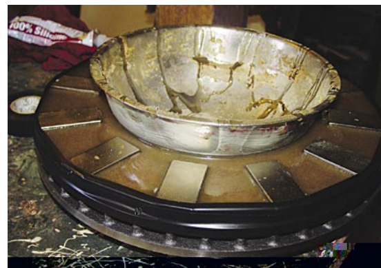
Photo 10: Molding the magnet rotors requires a stainless steel mixing bowl at the center and some duct tape around the edge to hold the resin.
