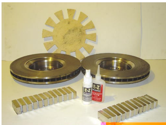
Photo 8: Magnet rotor materials include a plywood jig, two brake rotors, 24 magnets, and cyanoacrylate glue.
