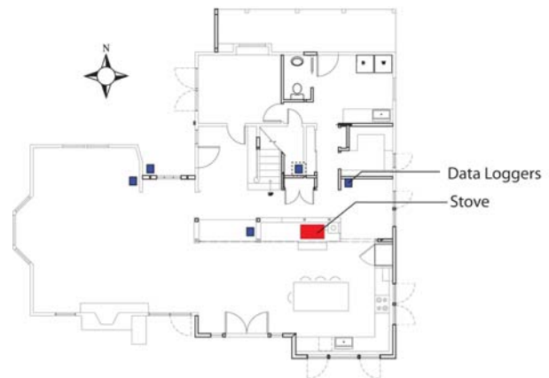
Figure 3. First floor plan of the Barkman residence showing the location of the contraflow masonry stove and data loggers.
